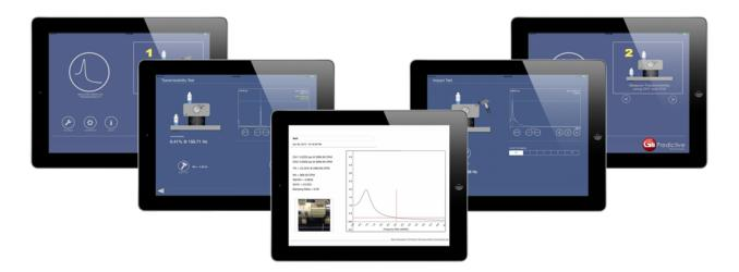
**Vibration Transmissibility** is an app that measures in real-time the percentage of vibrational energy that is being transmitted through a structure. It also plots the transmissibility curve of the system and indicates the operational point.
