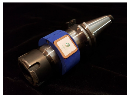
Embedded microtelemetry on CNC toolholder
