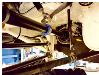
Suprocktech Microtelemetry in an automotive racing axle application
